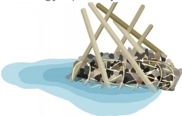
Place a structure in a river to change the flow, which scours and deepens the area around.
