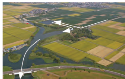
Fig. 4-7-5 River purification project (Measures for rivers draining into the Lake) (Purification by means such as temporary reservoirs and water plants before water drains from rivers into Lake Biwa)
