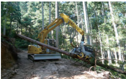
Fig. 3-14-2 Felling and transporting using high-performance forestry machinery
